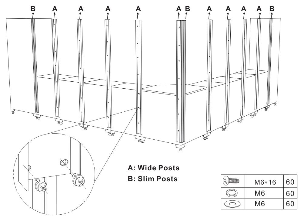
Step 3: Install 12 posts at the rear of the units by M6x16 bolts and make sure back panels are in middle of two cabinets.
