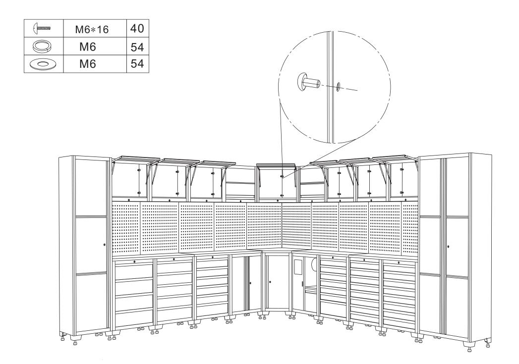
Step 7: Assemble 4 inner boards into the high cabinets, and 1 boards into the top cabinets.
