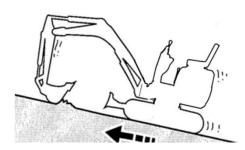
In event of traveling failure due to track slip while climbing up a slope, use the digging force of bucket arm to climb up the slope.
