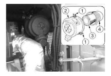
2. Loosen the clamp (1) and take out the dust collector (2).
