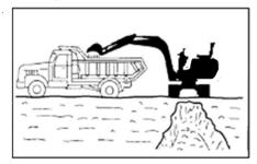
While loading soil into the cargo body of a truck, loading from the rear end of truck can load more soil easier than loading from the front end. In addition, the small angle slewing can be used to improve the efficiency.
