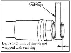
• While wrapping the screw plug with seal ring tape, thoroughly remove the used seal ring tap from the threads and clean the threads.
