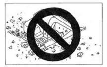
• Driving the machine on a riverbed or place with numerous pebbles can probably result in inclusion of pebbles in the tracks and the damage or falloff of tracks.
