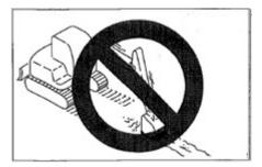
Do not insert the bucket into the ground or use the traveling force for digging.
