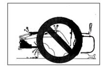
• Do not crush when the cylinder is fully extended or retracted (at travel end). Reserve at least 50mm travel.
