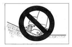
Please avoid driving the machine with one track on a slope or protrusion and the other track on level surface (In such case, this machine is inclined by 10° or more).
