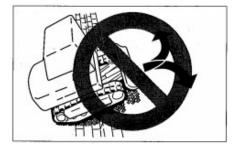
When driving over pebbles or large steps (≥20cm in depth, such as large rocks), climb on the steps in right angle and do not change route on steps.
