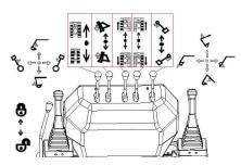
Use the right joystick to control the boom and bucket.
