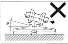
• In such case, the rubber tracks will fall off if the machine slews.
