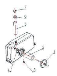
9. Loosen the bolt, remove the suction filter element (2), and clean it.
