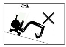
• If the bucket is fully loaded with material, avoid slewing towards the down slope direction. Otherwise, it will deteriorate the machine stability and probably result in rollover.
