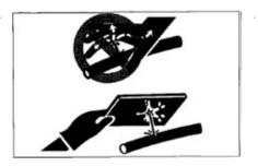
The high pressure of hydraulic oil can penetrate skin and eyes to cause serious injuries and blindness or even death. Please bear in mind that the hydraulic oil permeating from orifices is nearly invisible to naked eyes. While checking for leakage, wear goggles and thick gloves and protect the skin by paper boards or plywood to protect against the harms of spraying hydraulic oil.
