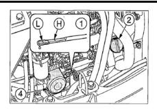
1. Open the engine hood and take out the oil filler port (2).
