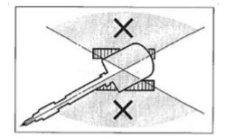
The machine is more vulnerable to rollover in lateral direction than longitudinal direction.
