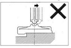
• In such case, the rubber tracks will fall off if the machine drives backward.
