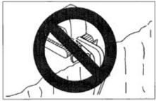
For deep digging operations, if the bulldozing blade is in the front, take cautions to prevent impacting the boom and bucket with bulldozing blade.
