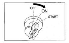
2. Turn the starter key to the ON position and hold it for about 60 seconds..
