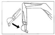
• With engine running at low speed, when the arm reaches a nearly vertical position, its retraction speed will drop shortly.
