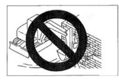
Do not use slewing force to dismantle walls or level ground. In addition, do not insert the bucket teeth into the ground during slewing. Otherwise the bucket working device will be damaged.
