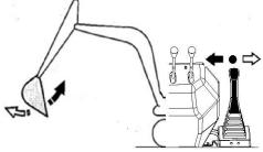
Load bucket: Push the right joystick left. Dump bucket: Push the right joystick right.
