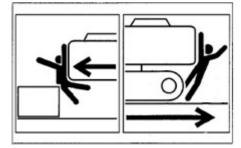
Verify the performance limits of machine. Set up a signaler at the road shoulders, narrow places, or vision-obstructed places.
