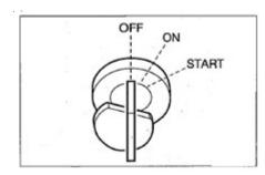
Important: Do not rotate the starter key from OFF to ON and then from ON to OFF repeatedly within a short time, otherwise it will probably result in engine malfunction.
