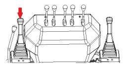
This button is used for the operation of attachments that require hydraulic power such as breakers.
