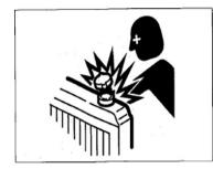
Do not disassemble the radiator cap or drainage plug when the coolant is hot. Stop the engine and wait for the engine and coolant to cool down. Slowly loosen the radiator cap to relieve the internal pressure and then take it out.
