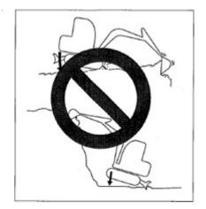
Using additional tension onto the machine will shorten the life of machine. During digging, use the hydraulic force of cylinders by shallow depth and large travel.
