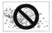
Driving and steering the machine on gravels, rough and hard rocks, steel beams, or scrap irons or near the edges of steel plates will damage the rubber tracks.
