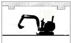
During operations under bridges, in tunnels, near cables, or indoors, guard the boom and bucket arm against impact with any overhead object.
