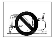
Do not crush when the bucket arm is perpendicular to the ground.
