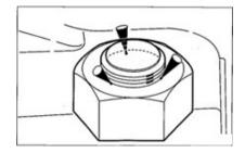
Rivet the bolt by a press or perform threepoint welding at the threaded portion (Nut end).
