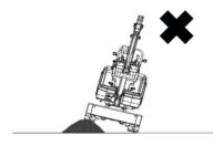
Driving the machine over obstacles (Including rocks and stumps) will probably apply high load onto the machine body and damage the machine. Avoid driving over obstacles whenever possible. If it's necessary to drive over obstacles, close the bucket working device to the ground, drive the machine at low speed, and drive the machine in such manner that the obstacles are in the middle of tracks.
