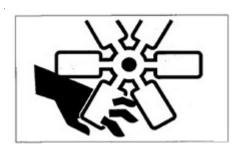
Keep away from all rotating and motion parts. The entanglement of hands or tools into rotating or moving parts will probably cause accidents of serious injuries or even deaths. The tools or other objects fallen or inserted into the fan or fan belt will be crushed or cut. Never throw or insert any object into fan or fan belt.
