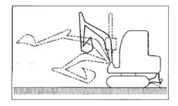
Slowly telescope all cylinders for several times under no-load condition.
