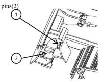
Rotate the extension plate around the pins for 180°.
