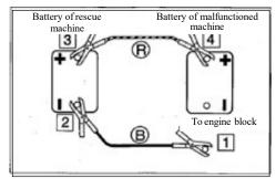
Disconnect the clamp of jumper cable (B) from the engine support of malfunctioned machine.
