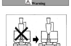
Do not use breaking hammer when the track width becomes narrower.
