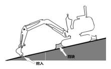
• If it's necessary to park the machine or tilt the machine on a slope, securely park the machine and block the machine against movement.
