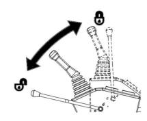
1. Fully lower the safety lock lever to release the lock.
