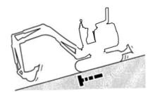
While driving down a slope, the brake applies braking automatically after the traveling joystick returns to neutral position.
