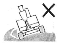
Do not access any soft ground area. This will probably result in inclination of machine due to dead weight to cause rollover or ground entrapment.
