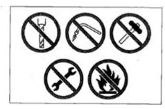
Take special cautions while handling the high pressure nitrogen stored in the tank. The improper handling will probably result in explosion of nitrogen to cause serious injuries. Please strictly abide by the following safety measures:
