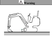
• Stop the machine on a level, solid, and safe ground. Set the parking device.
