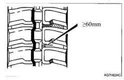
If the cracking length is  $\geq$ 60mm, repair. If the wire rope is visible, repair as soon as possible, regardless of the cracking length.
