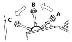
Used to control engine speed.
