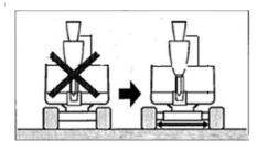
Always operate the machine with extended track width of 950mm, in order to improve the machine stability to the maximum extent. Operating the machine with narrow track width (800mm) will probably result in rollover of machine due to poor stability.
