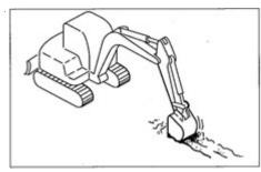
Install a bucket suitable for digging of ditches, adjust the tracks to be parallel with the ditch to be dug, in order to improve the working efficiency. While digging a wide ditch, dig the side faces and then the middle area.
