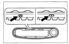
1. For rubber tracks, adjust the marking "M" at the joints to the top center of track frame.
