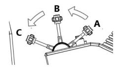
1. Pull the accelerator joystick to neutral position. Then, run the engine at medium
