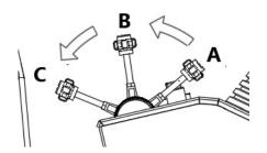
1. Pull the accelerator joystick to increase the engine speed.
