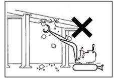
Do not perform demolition operations above your head. There is a falling damage of damaged parts or collapse danger of building to cause serious harms or destruction.
