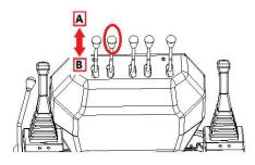
Use this joystick to operate the bulldozing blade.
