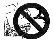
• While reversing up a slope, do not change direction at the start point of slope.
