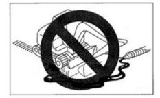
• Keep the tracks away from the adhesion of fuel, lubricating oil, salt, and chemical solvent. These substances will probably corrode the welds of track steel cores to cause rusting or falloff. Such substances adhered onto the tracks shall be immediately removed by water.
