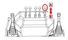
This lever controls the hydraulic oil flow and direction in the auxiliary hydraulic circuit.
