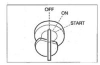
Insert the key into start switch, rotate to ON position, and then check as below:
