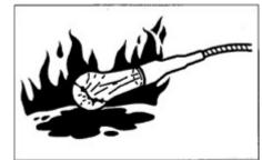
While checking the fuel, lubricating oil, coolant, and battery electrolyte, please use explosion- proof lamps to prevent fire and explosion. Otherwise, it will probably result in explosion to cause serious injury accidents.
