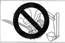
Impacting the bulldozing blade with rock will damage the bulldozing blade and bulldozing blade cylinder.
