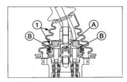
1.Remove the lower base part of the sheath (1) and turn it up.
