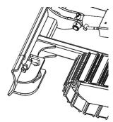
3. Install the pins and tighten the bolts.
