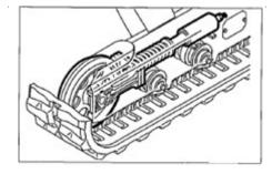
The track pensioner is installed with a high strength spring. If the track pensioner is disassembled carelessly, the spring will spring out to cause serious injuries. Do not disassemble the track pensioner.
