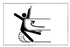
Never place your hand, foot, or other body parts between the superstructure and chassis or tracks, between machine body and working device, or between cylinder and motion parts. During movement of machine, these clearances will change to probably cause serious injuries or deaths.
