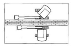
As shown in the diagram, dig the side ditch by swing function of boom.
