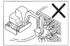
Do not perform the demolition operations by the impact force of bucket working device. The splashed material fragments and the damaged bucket working device have a danger of serious harms.
