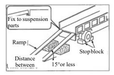
The machine will probably roll over or fall off during loading and unloading. Ensure to take the following safety measures: Select a solid and level ground and keep a sufficient spacing from the road curb. Fix the ramps of sufficient strength and dimensions to the cargo body of truck. The inclination of the ramps shall not exceed 15°. If the ramps deflect downward excessively, please support the ramps by supports or cushion
