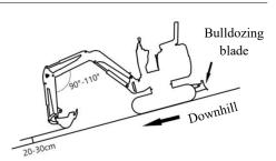
Keep the driver seat facing towards the up slope direction while climbing up a slope. Keep the driver seat facing towards the down slope direction during down slope traveling. In both cases, pay special attention to the ground ahead of the machine during traveling.
