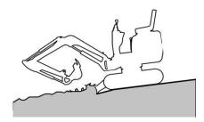
This bulldozing blade is designed for simple bulldozing operations. Do not use the bulldozing blade for deep digging. Otherwise, the bulldozing blade and the under frame will probably be damaged.
