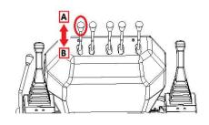
3. Push the lever forward to increase the width of the chassis to 950 mm.
