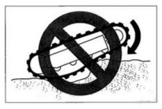
• Do not change the direction when the tracks are loose as shown in the diagram.
