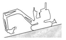
If the engine stops while driving down a slope, shift the traveling joystick to neutral position, stop the machine, and then restart the engine.
