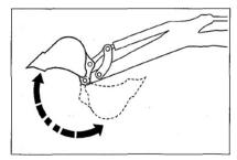
2. Operate the bucket cylinder to an end and hold.
