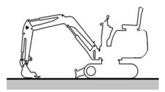
• Stop the machine on a level, solid, and safe ground. Set the parking device.
