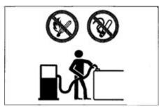
The smoking and open fire are prohibited during refueling and near the refueling point. Do not disassemble the fuel tank cap or refuel while the engine is running or is not cooled down. Do not splash fuel to any high temperature surface of machine.
