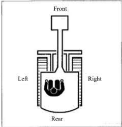
The front, rear, left, and right of the machine indicated in this manual are based on the status sitting in the driver seat, with the bulldozing blade visible in the front.
