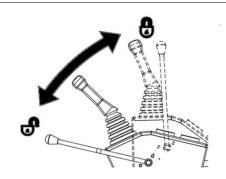
This device is functioned to lock the operations of bucket working device and machine slewing. When pushing the lever forward, except for the walking lever, the other levers cannot work
