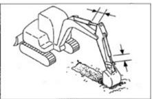
Do not extend any hydraulic cylinder to the end. Reserve an allowance during operations.
