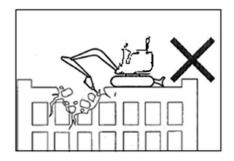
• Do not perform demolition operations beneath the machine. There is a possible falling danger of machine when the ground becomes unstable.  Before the operations on the top of any building or other structure, check the strength and structure. It will cause serious harms or destruction if the building or structure collapses.
