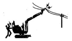
Never close any part or loaded material of machine to high-voltage cables, unless all safety measures specified by local and national authorities are already taken. There is a danger of electric shock and death when any person approaches to the machine that is discharging electric spark or is near or in contact with power supply.
