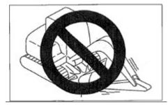
While retracting the bucket working device, take cautions not to impact the bucket with bulldozing blade.
