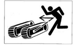
In the track pensioner, the grease is injected under high pressure. If the tension is not adjusted by the following designated procedure, the grease relief valve will probably fly out to cause injuries.
