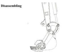
1. Lower the bucket steadily onto the ground as shown in above diagram.
