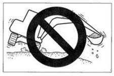
• The rubber tracks are not as stable as steel tracks, as they are completely made of rubber. Take special cautions during the lateral slewing and swing.
