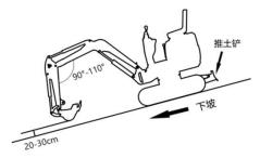
While driving down a 15° or higher slope, reduce the engine speed and maintain the machine posture shown in above diagram.
