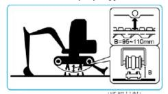
20. Keep the boom and bulldozing blade separated. While lowering the boom, take cautions not to touch the boom with bulldozing blade.
