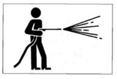
Please clean the machine before maintenance. Stop the engine before cleaning the machine. Cover the electric parts against water ingress. The water ingress into the electric parts will probably result in short-circuit or malfunction. Do not clean the battery, electronic control units, sensors, connector, or cab by water or steam.
