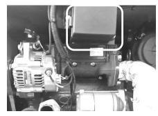
If the machine does not start after turning the start switch to the ON position, it may be that the starting power fuse has blown. Open the service cover and check. If the fuse has blown, please contact your sales or service agent.
